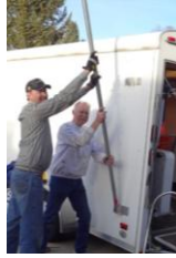
Then lock pole into the brackets on side of trailer.
